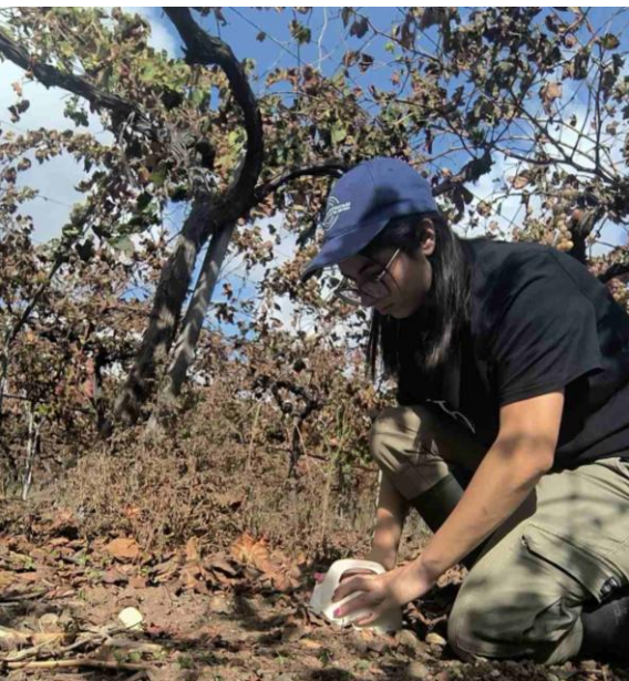
Quantification of CO 2 respiration using a chamber in vine plot
